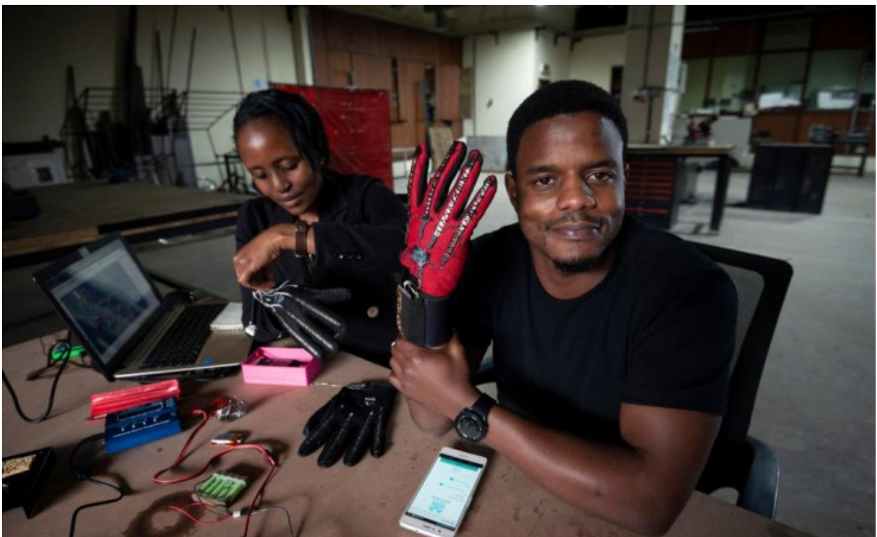
Roy Allela (R) with one of the smart gloves he has invented. Dubbed Sign-IO, the gloves help convert sign language to speech. [Photo/ BrettEloff/RoyalAcademyofEngineering]
